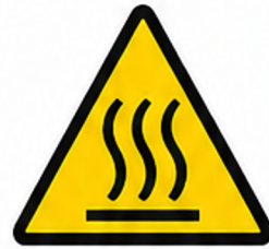
Hot Surface Burn Hazard
